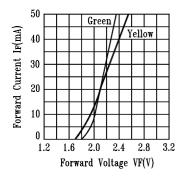
Fig.2 Forward Current vs. Forward Voltage
