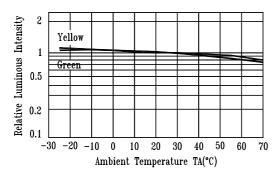
Fig.5 Luminous Intensity vs. Ambient Temperature
