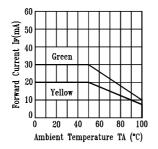
Fig.3 Forward Current Derating Curve
