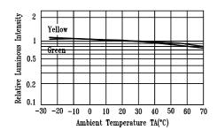
Fig.5 Luminous Intensity vs. Ambient Temperature
