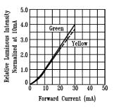
Fig.4 Relative Luminous Intensity vs. Forward Current
