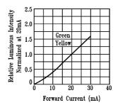
Fig.4 Relative Luminous Intensity vs. Forward Current
