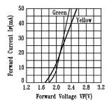
Fig.2 Forward Current vs. Forward Voltage
