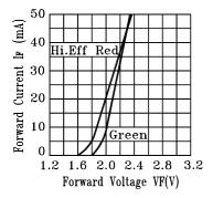
Fig.2 Forward Current vs. Forward Voltage
