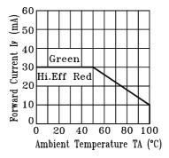
Fig.3 Forward Current Derating Curve
