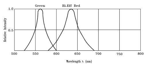
Fig.1 Relative Intensity vs. Wavelength
