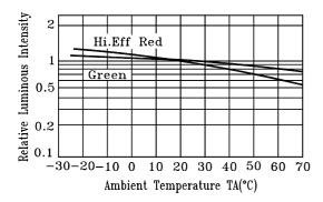
Fig.5 Luminous Intensity vs. Ambient Temperature
