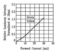
Fig.4 Relative Luminous Intensity vs. Forward Current
