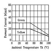
Fig.3 Forward Current Derating Curve
