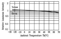
Fig.5 Luminous Intensity vs. Ambient Temperature
