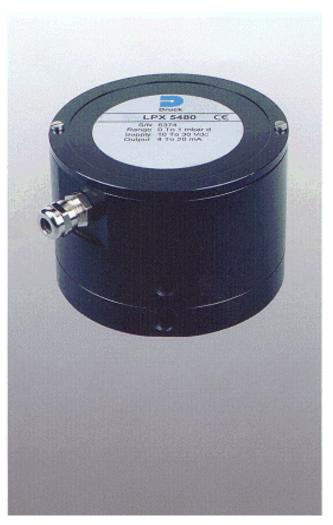
The LPM/LPX 5000 Series Differential pressure transducers/transmitters are rugged, watertight (IP66/NEMA 4: when cover is in place and cable is installed properly) for accurate measurement of differential or relative pressures of gases and liquids, in the ranges between the full scale ranges of 0.0075psid (0.2"WCD) and 15 PSID in both unidirectional and bidirectional modes with line pressures of up to 300 psig.
