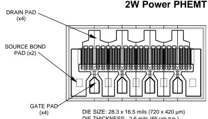
DIE THICKNESS: 2.6 mils (65 µm typ.)
