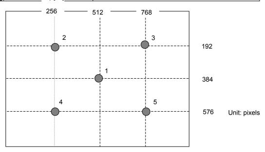
Note 1: Average brightness is the average of brightness value at location 1 to 5 with all pixels displaying white. (C) Copyright Acer Display Technology, Inc.
