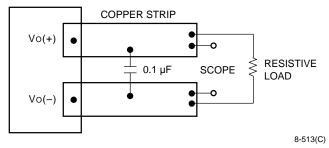
Note: Use a 0.1 µF ceramic capacitor. Scope measurement should be made using a BNC socket. Position the load between 50.8 mm and 76.2 mm (2 in. and 3 in.) from the module.
