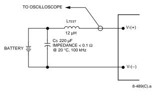
Note: Input reflected-ripple current is measured with a simulated source impedance of 12  $\mu$ H. Capacitor Cs offsets possible battery impedance. Current is measured at the input of the module.
