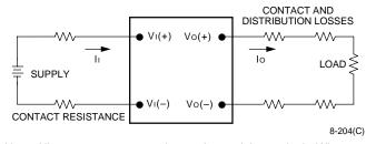
Note: All measurements are taken at the module terminals. When socketing, place Kelvin connections at module terminals to avoid measurement errors due to socket contact resistance.
