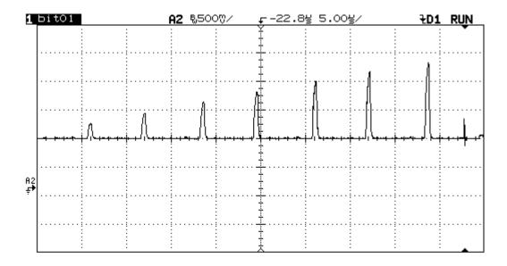
LIS-128 running at 40Mhz pixel read rate or 148,000 frames/sec. Illustrates non destructive read for seven frames.
