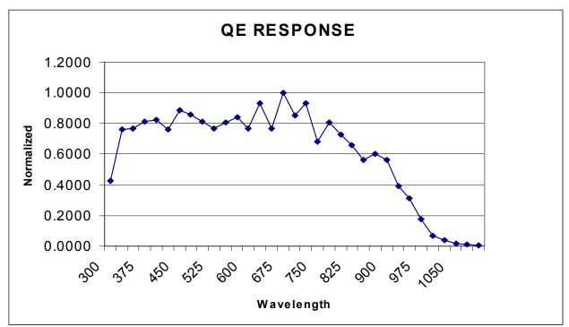
Note: Data below 350nm not measured, but device is sensitive to 200 nm. Shown for un-encapsulated device.
