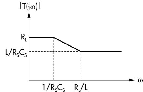
FIGURE 12 — Sensor Gain
