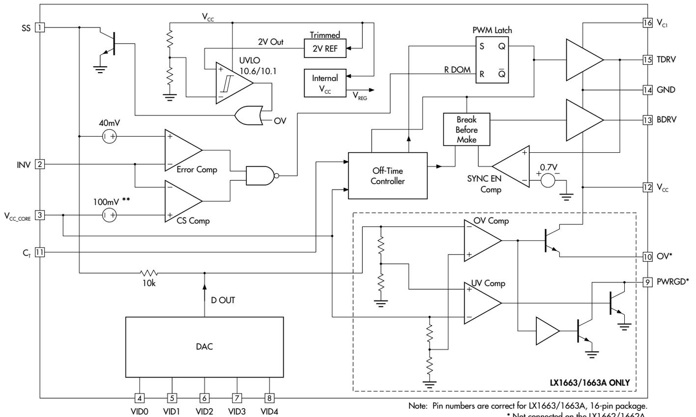
FIGURE 5 — Block Diagram
