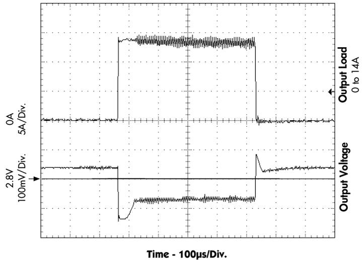
**FIGURE 1** — Output Transient Response
