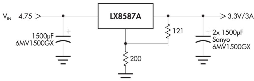
The output capacitors must be low ESR and low ESL type for good transient response.
