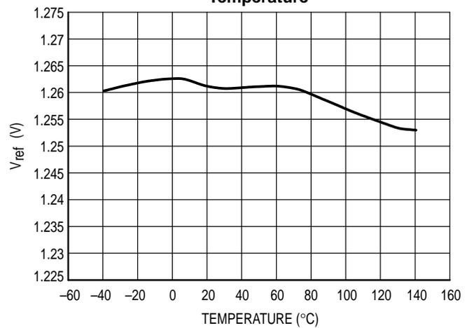
**Figure 5. LT1585A-1.5 Output Voltage vs Temperature**
