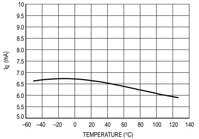
Figure 7. LT1585A Adjust Pin Current vs Temperature
