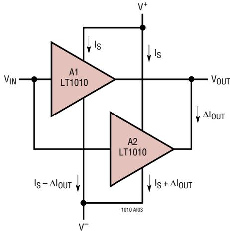
Output load current will be divided based on the output resistance of the individual buffers. Therefore, the available output current will not quite be doubled unless output resistances are matched. As for offset voltage, the  $25^\circ C$  limits should be used for worst-case calculations.
