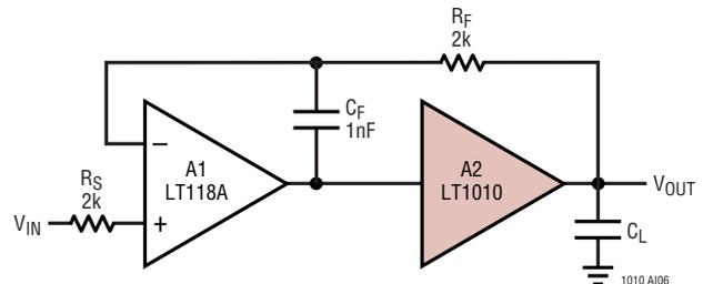
The follower configuration is unique in that capacitive load isolation is obtained without a reduction in small-signal bandwidth, although the output impedance of the buffer comes into play at high frequencies. The precision unity-gain buffer above has a 10MHz bandwidth without capacitive loading, yet it is stable for all load capacitance to over  $0.3\mu F$ , again determined by  $R_F C_F$ .
