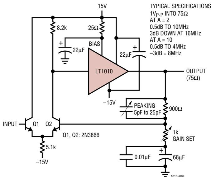
stage. Feedback is arranged in the conventional manner, although the  $68\mu F-0.01\mu F$  combination limits DC gain to unity for all gain settings. For applications sensitive to NTSC requirements, dropping the  $25\Omega$  output stage bias value will aid performance.
