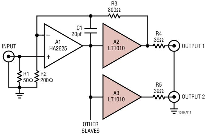
The 50Ω video line splitter here puts feedback on one buffer with the others slaved. Offset and gain accuracy of slaves depend on their matching with master.
