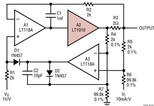
enables the current regulator to get control of the output current from the buffer current limit within a microsecond for an instantaneous short.
