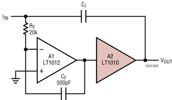
If the integrating capacitor must be driven from the buffer output, the circuit above can be used to provide capacitive load isolation. As before, the stability with large capacitive loads is determined by  $R_F C_F$ .
