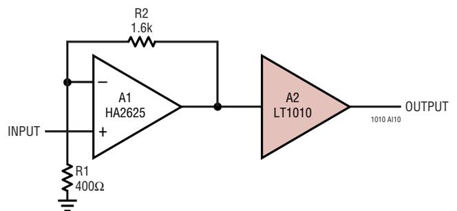
Putting the buffer outside the feedback loop as shown here will give capacitive load isolation, with large output capacitors only reducing bandwidth. Buffer offset, referred to the op amp input, is divided by the gain. If the load resistance is known, gain error is determined by the output resistance tolerance. Distortion is low.
