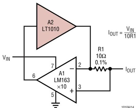
Output resistances of several megohms can be obtained with both circuits. This is impressive considering the ±150mA output capability. High frequency output characteristics will depend on the bandwidth and slew rate of the amplifiers. Both these circuits have an equivalent output capacitance of about 30nF.
