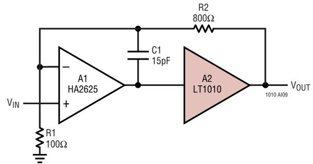
This shows the buffer being used with a wideband amplifier that is not unity-gain stable. In this case,  $C_1$  cannot be used to isolate large capacitive loads. Instead, it has an optimum value for a limited range of load capacitances.
