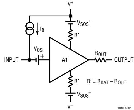
Loaded voltage gain can be determined from the unloaded gain,  $A_V$ , the output resistance,  $R_{OUT}$ , and the load resistance,  $R_L$ , using:
