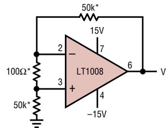
\* RESISTORS MUST HAVE LOW THERMOELECTRIC POTENTIAL
