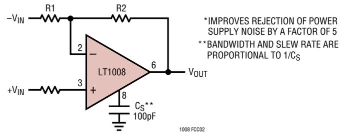
FOR  $\frac{R_2}{R_1} > 200$ , NO EXTERNAL FREQUENCY COMPENSATION IS NECESSARY
