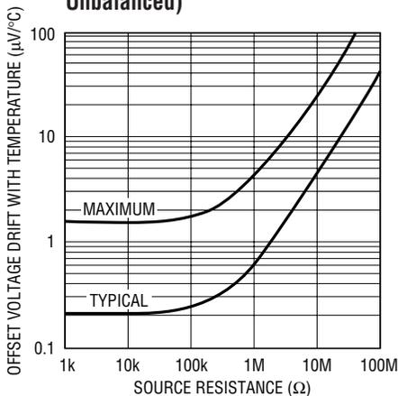
Offset Voltage vs Source Resistance (Balanced or Unbalanced)
