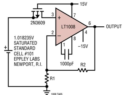
THE TYPICAL 30pA BIAS CURRENT OF THE LT1008 WILL DEGRADE THE STANDARD CELL BY ONLY 1ppm/YEAR. NOISE IS A FRACTION OF A ppm. UNPROTECTED GATE MOSFET ISOLATES STANDARD CELL ON POWER DOWN
