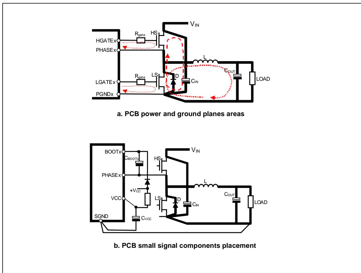
Fig. 15a shows the details of the power connections involved and the current loops. The input capacitance ( $C_{IN}$ ), or at least a portion of the total capacitance needed, has to be placed close to the power section in order to eliminate the stray inductance generated by the copper traces. Low ESR and ESL capacitors are required.
