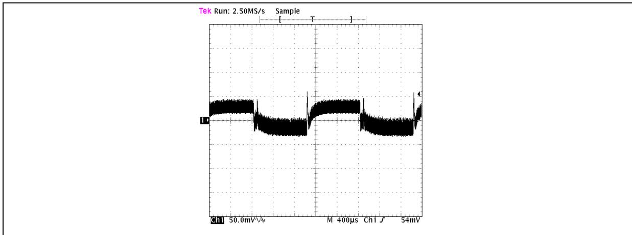
Figure 30 shows the system response to a VID transient from 1.200V to 0.800V and vice versa at minimum load (3A).
