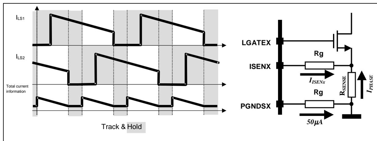
This circuit sources a constant 50µA current from the PGNDsX pin and keeps the pins ISENx and PGNDsX at the same voltage. Referring to figure 4, the current that flows in the ISENx pin is then given by the following equation:
