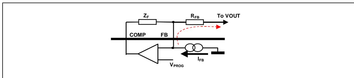
The feedback current is equal to  $50\mu A$  at nominal full load ( $I_{FB} = I_{INFO1} + I_{INFO2}$ ) and  $70\mu A$  at the OC intervention threshold, so the maximum output voltage deviation is equal to:
