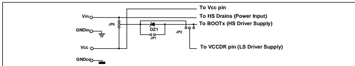
Two main configurations can be distinguished: Single Supply ( $V_{CC}=V_{IN}=12V$ ) and Double Supply ( $V_{CC}=12V$   $V_{IN}=5V$  or different).
