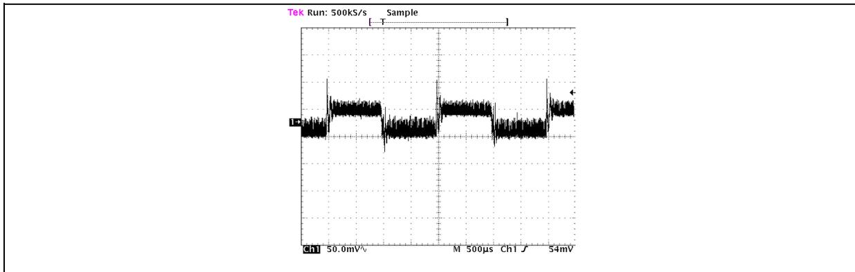
Figure 26 shows the system response to a VID transient from 1.200V to 0.800V and vice versa at minimum load (3A).
