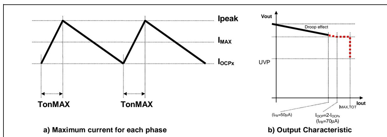
It can be observed that the peak current ( $I_{peak}$ ) is greater than the  $I_{OCPx}$  but it can be determined as follow:
