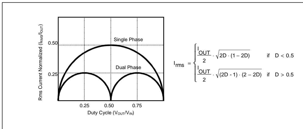
It can be observed that the input rms value is one half of the single-phase equivalent input current in the worst case condition that happens for  $D = 0.25$  and  $D = 0.75$ .
