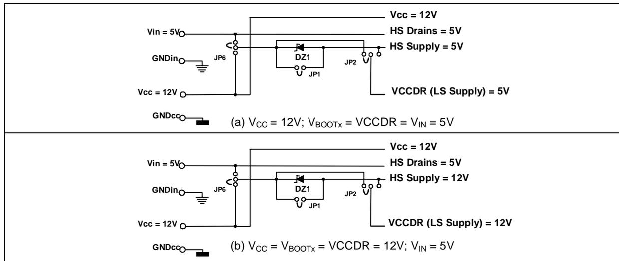
**Figure 21. Jumpers configuration: Single Supply**
