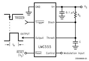
FIGURE 8. Pulse Width Modulator
