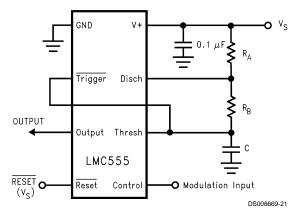
FIGURE 10. Pulse Position Modulator
