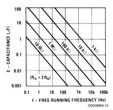
FIGURE 6. Free Running Frequency
