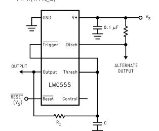
FIGURE 12. 50% Duty Cycle Oscillator
