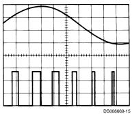
$V_{CC} = 5V$ Top Trace: Modulation 1V/Div. TIME = 0.2 ms/Div. Bottom Trace: Output Voltage 2V/Div.  $R_A = 9.1 \text{ k}\Omega$
