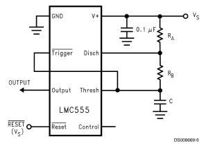
FIGURE 4. Astable (Variable Duty Cycle Oscillator)
