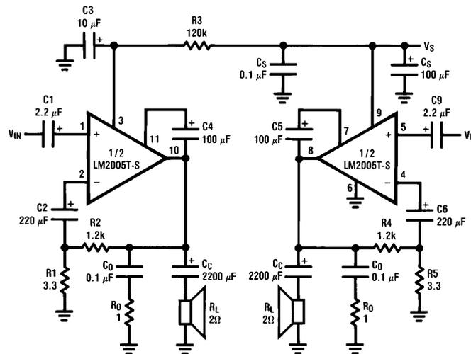
FIGURE 2. 10W/Channel Stereo Amplifier Application and Test Circuit
