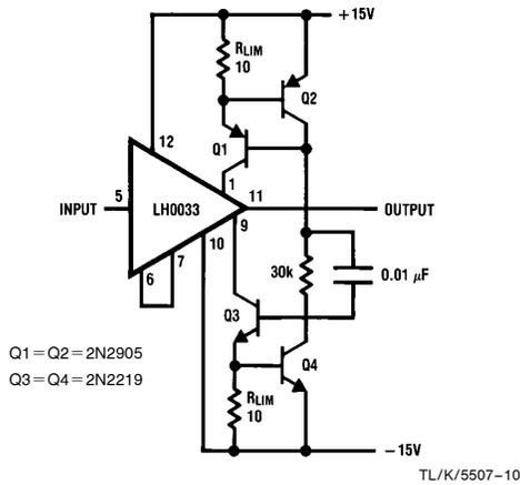
FIGURE 5. LH0033 Current Limiting Using Current Sources
