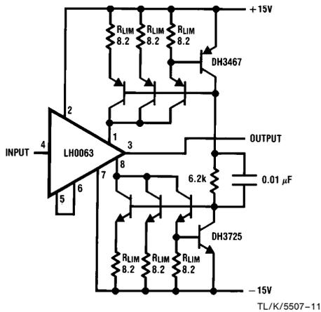
FIGURE 6. LH0063 Current Limiting Using Current Sources
