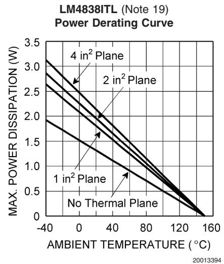
**Note 19:** These curves show the thermal dissipation of the LM4838ITL at different ambient temperatures with a thermal plane of size shown on an outside PCB layer using 1oz. copper.
