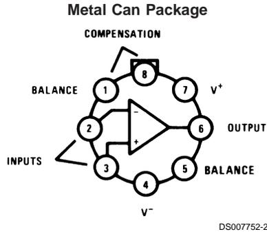
Note: Pin 4 connected to case.
