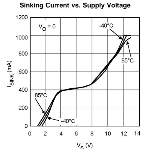
**Typical Performance Characteristics** At  $T_J = 25^\circ\text{C}$ ,  $R_F = 470\Omega$  gain = +2,  $R_L = 100\Omega$ . Unless otherwise specified. (Continued)
