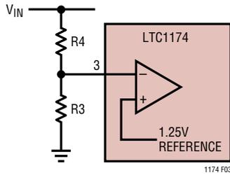
Figure 3. Low-Battery Comparator
