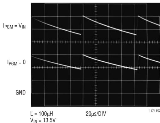
Figure 2. Inductor's Current with Output Shorted
