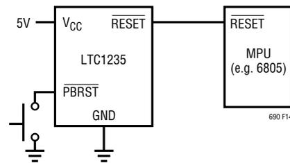
Figure 14. The External Push-Button Reset with the LTC1235
