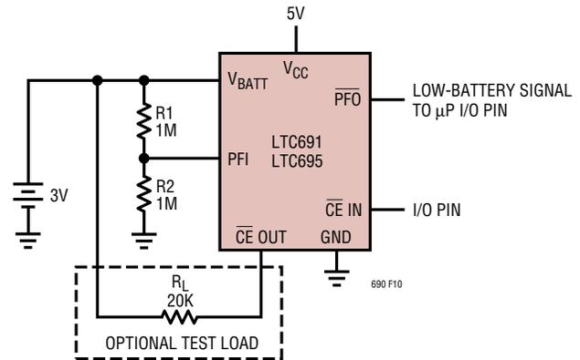
Figure 10. Back-Up Battery Monitor with Optional Test Load
