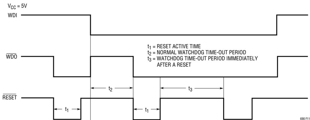
Figure 11. Watchdog Time-Out Period and Reset Active Time
