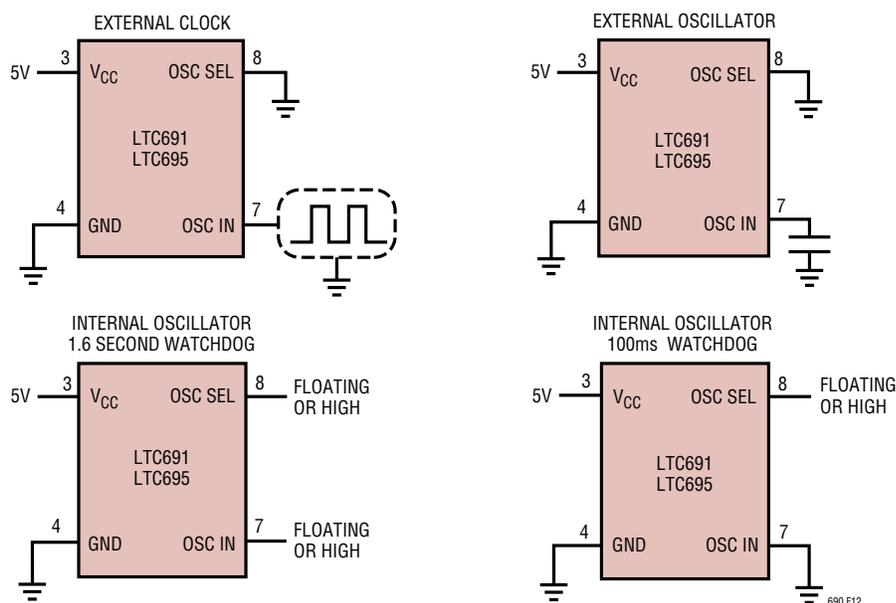
Figure 12. Oscillator Configurations
