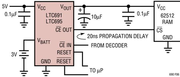
Figure 6. A Typical Nonvolatile CMOS RAM Application
