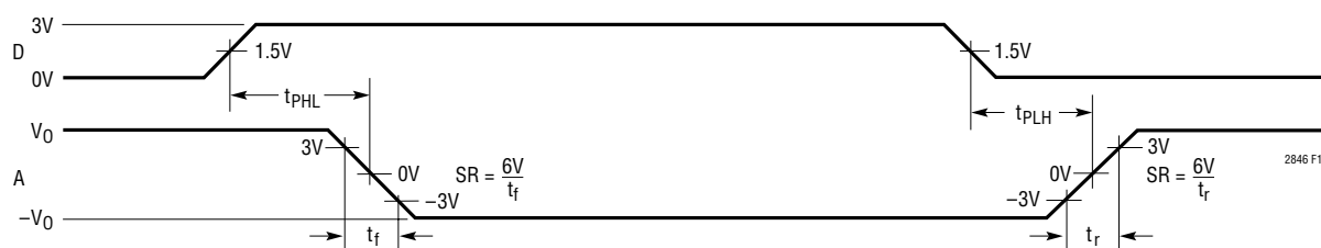
Figure 15. V.28 Driver Propagation Delays
