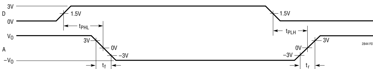
Figure 7. V.10, V.28 Driver Propagation Delays
