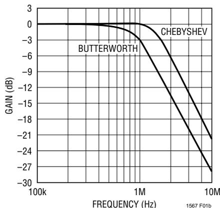
GAIN IS MEASURED TO EITHER OUTPUT ALONE.
