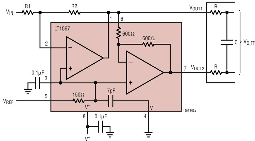
$$V_{OUT1} = -\frac{R2}{R1} \cdot V_{IN} + \left(\frac{R2}{R1} + 1\right) \cdot V_{REF} \quad V_{OUT2} = -V_{OUT1} + 2 \cdot V_{REF}$$
