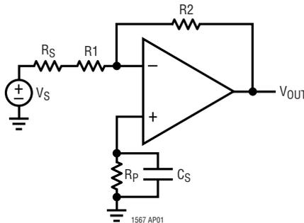
NOISE AT  $V_{OUT}$  IN  $V_{RMS} = V_{ON}$  IN  $V/\sqrt{Hz} \cdot \sqrt{f_{NBW}}$
