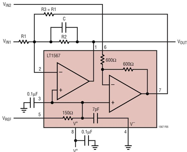
WITH R3 AND R1 EQUAL,  $V_{OUT} = V_{REF} + \left(\frac{R2}{R1}\right) (V_{IN2} - V_{IN1})$
