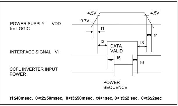
\* Set 0 Volt Vi(t) ≤ V<sub>DD</sub>(t) Here Vi(t), V<sub>DD</sub>(t) indicate the transitive state of Vi, V<sub>DD</sub> when power supply is turned ON or OFF
