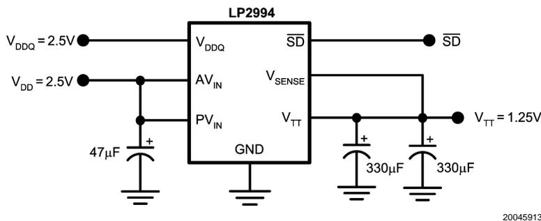
FIGURE 13. Typical SSTL-2 Application Circuit for Motherboards
