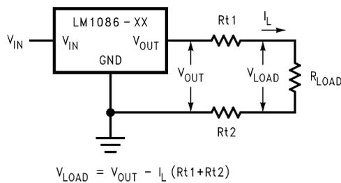
$$V_{LOAD} = V_{OUT} - I_L (R_{t1} + R_{t2})$$
