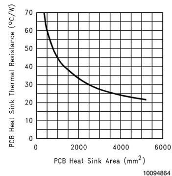
FIGURE 7. Heat sink thermal Resistance vs. Area
