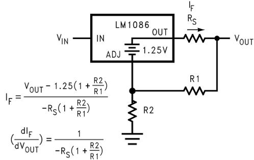
$$I_F = \frac{V_{OUT} - 1.25(1 + \frac{R_2}{R_1})}{-R_S(1 + \frac{R_2}{R_1})}$$
