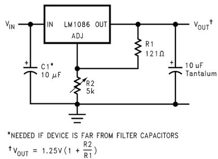
\*NEEDED IF DEVICE IS FAR FROM FILTER CAPACITORS
