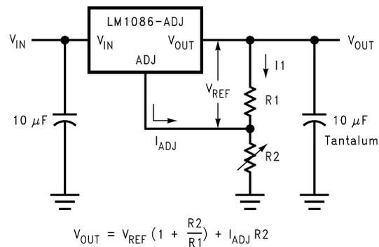
$$V_{OUT} = V_{REF} \left( 1 + \frac{R_2}{R_1} \right) + I_{ADJ} R_2$$
