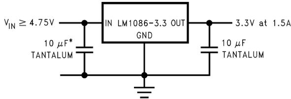
\*MAY BE OMITTED IF INPUT SUPPLY IS WELL BYPASSED WITHIN 2" OF THE LM1086
