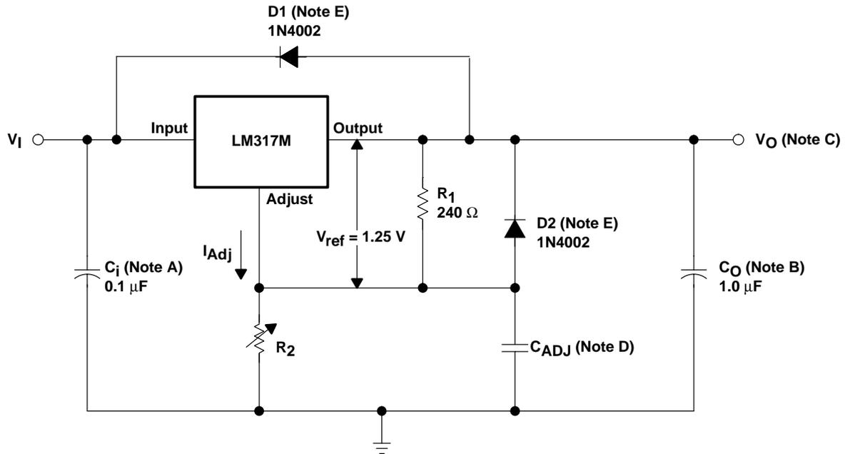
NOTES: A.  $C_i$  is not required, but is recommended, particularly if the regulator is not in close proximity to the power-supply filter capacitors. A 0.1- $\mu$ F disc or 1- $\mu$ F tantalum provides sufficient bypassing for most applications, especially when adjustment and output capacitors are used.
