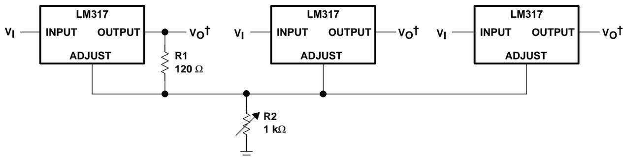
† Minimum load current from each output is 10 mA. All output voltages are within 200 mV of each other.
