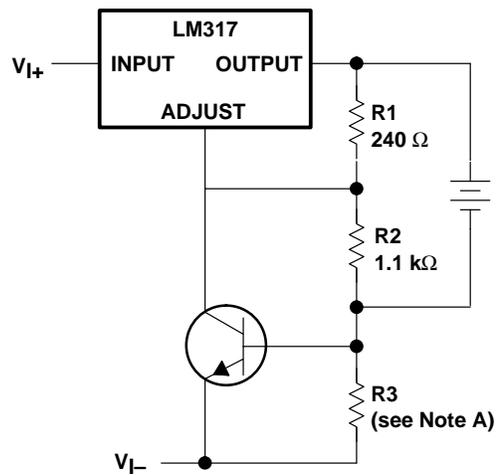
NOTE A: R3 sets the peak current (0.6 A for a 1-Ω resistor).
