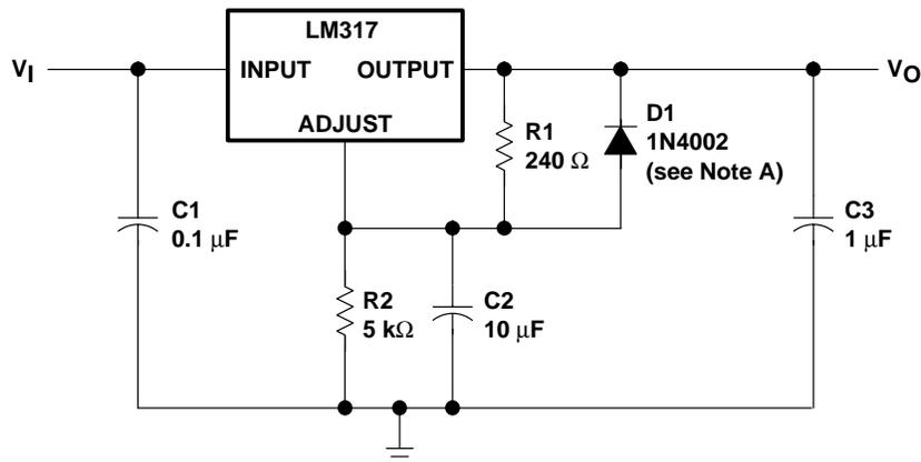
NOTE A: D1 discharges C2 if the output is shorted to ground.
