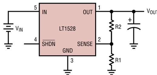
$$V_{OUT} = 3.3V \left( 1 + \frac{R_2}{R_1} \right) + (I_{SENSE} + R_2)$$
