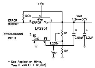
\*\* Drive with TTL high to shut down. Ground or leave open if shutdown feature is not to be used.
