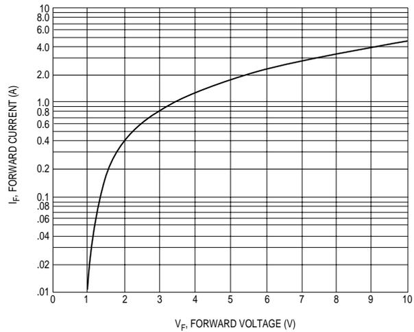
**Figure 4. Forward Voltage vs. Forward Current**
