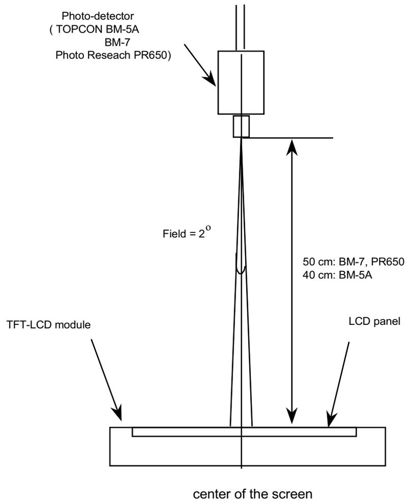
Optical characteristics measurement setup
