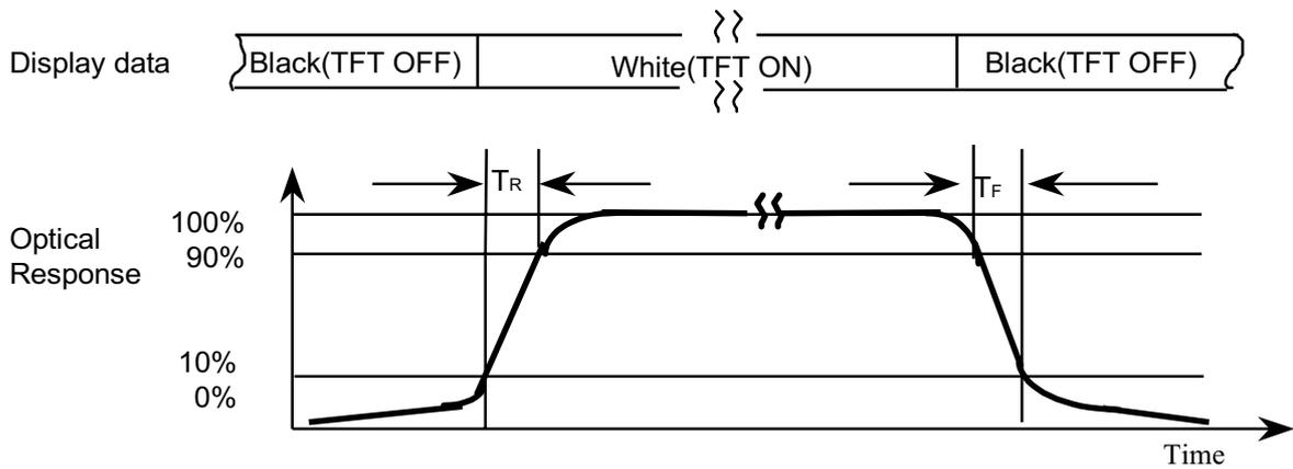
Note 4) After stabilizing and leaving the panel alone at a given temperature for 30 min , the measurement should be executed. Measurement should be executed in a stable, windless, and dark room. 30 min after lighting the back-light. This should be measured in the center of screen. Each lamp current : 6.5mA (Refer to the note(1) in the page 10 for more information.) Environment condition :  $T_a = 25^{\circ}\text{C} \pm 2^{\circ}\text{C}$
