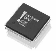
The LS800 Internet TV System-on-Chip has advanced features such as Picture-In-Picture, external device support and a softmodem.
