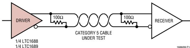
Figure 14. Test Circuit for Cable Speed Evaluation
