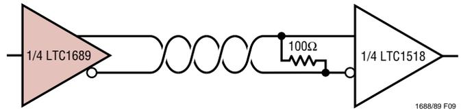
Figure 9. Point-to-Point Transmission
