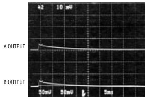
Figure 7. Common Mode Charge Injection During Hot Swapping
