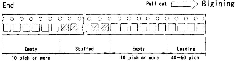
(2) Cover tape strength against peeling:  $F=0.1\sim0.8N$  ( $\theta = 10^\circ$  or less)
