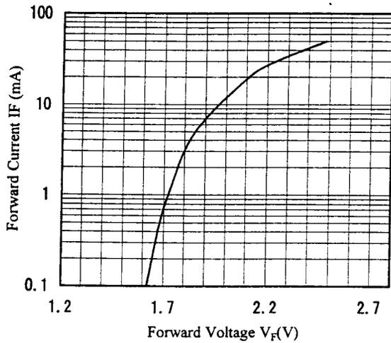
Forward Current vs. Forward Voltage ( $T_a=25^\circ\text{C}$ )
