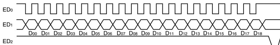
The serial data ED1 is shifted by ED0 and is latched at the rising edge of ED2.
