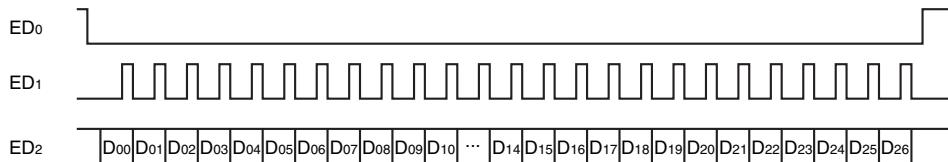
The data on ED2 is latched in the register at the rising edge of ED1.
