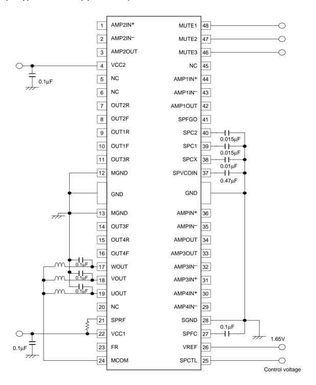
Note: The values of external components shown here are provided for reference purposes and differ from the optimal values, which depend on the motors actually used, in any particular application.
