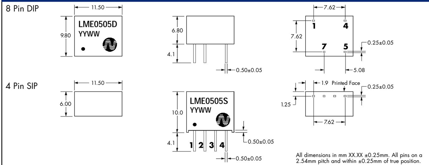
All dimensions in mm XX.XX ±0.25mm. All pins on a 2.54mm pitch and within ±0.25mm of true position.
