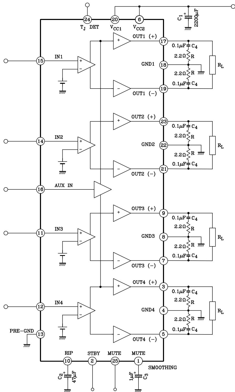
(Note) Please be careful that the pin ① and the pin ②5 are exchanged in comparison with before data sheet, and the non-inverse output and the inverse output are exchanged, too.
