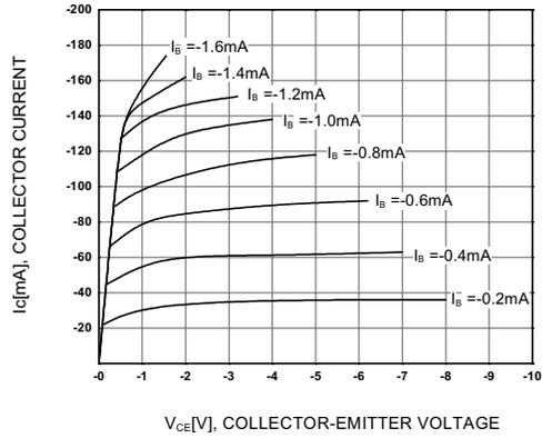
Figure 1. Static Characteristic
