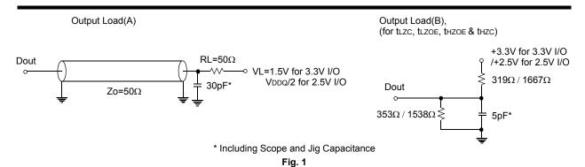
AC TIMING CHARACTERISTICS(VDD=3.3V+0.165V/-0.165V, TA=0 to 70°C)
