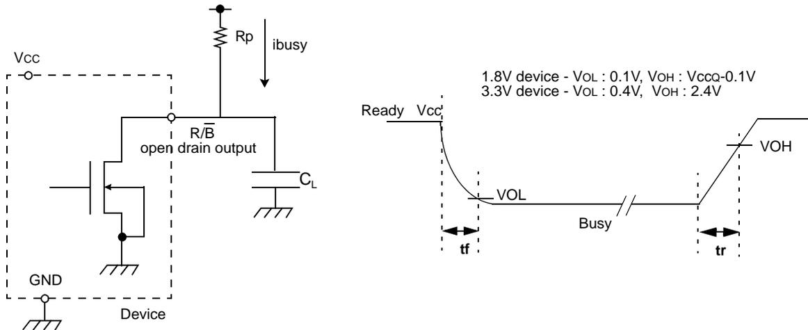
Figure 17. Rp vs tr ,tf & Rp vs i<sub>busy</sub>
