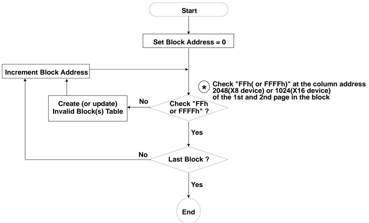
**Figure 3. Flow chart to create invalid block table.**
