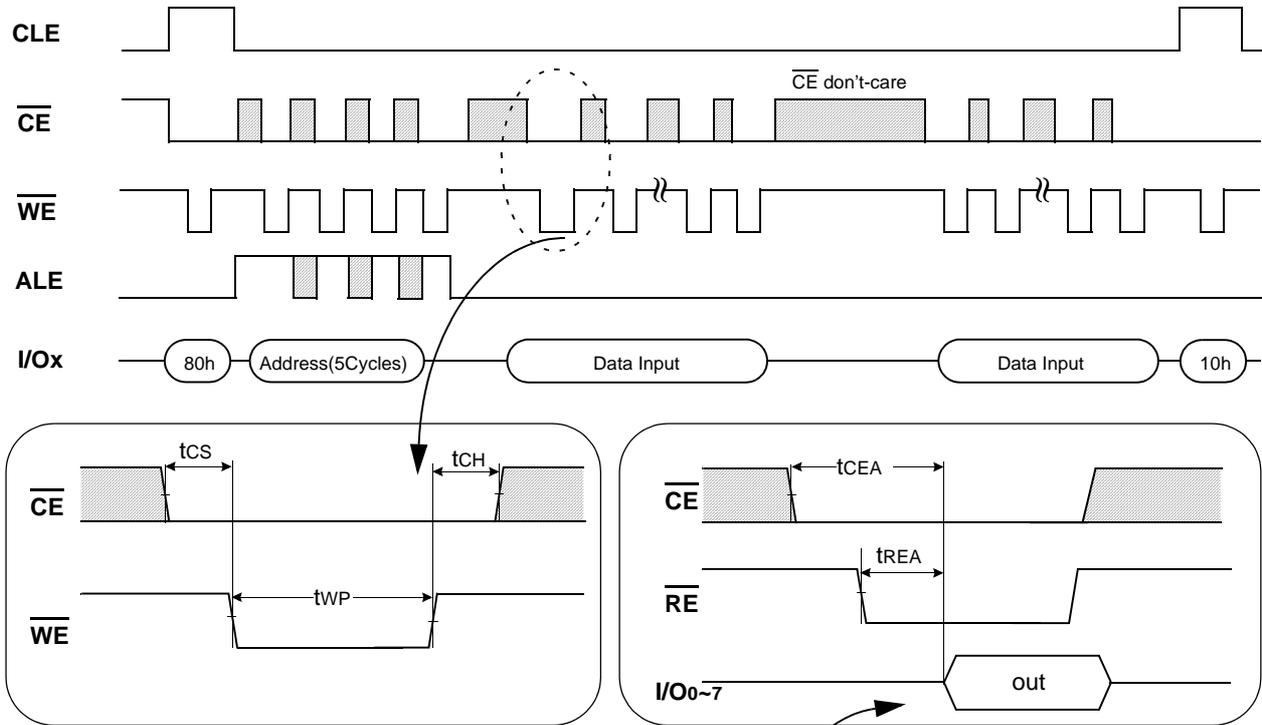
**Figure 5. Read Operation with  $\overline{CE}$  don't-care.**
