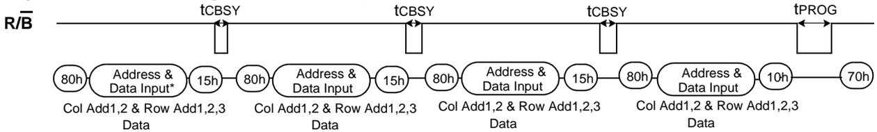
**NOTE :** Since programming the last page does not employ caching, the program time has to be that of Page Program. However, if the previous program cycle with the cache data has not finished, the actual program cycle of the last page is initiated only after completion of the previous cycle, which can be expressed as the following formula.
