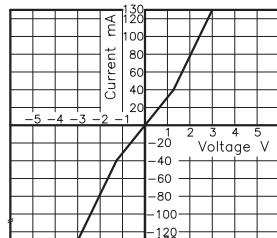
**Fig.9** Off state leakage current
