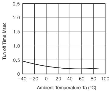
**Fig.5** LED operate vs. ambient temperature
