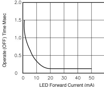
**Fig.11** LED forward current vs. reverse (ON) time Across terminals 3 and 4 pin;
