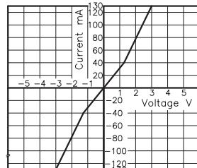
**Fig.9** Off state leakage current
